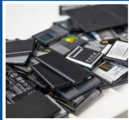
Before recycling, hazardous or noxious substances such as batteries, fluorescent tubes and radiation sources are removed from the equipment. This multi-stage processing results in high-quality recycled raw materials that are sold to various industries.
